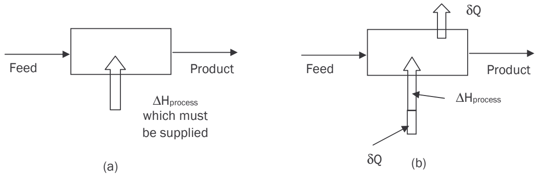
Figure 5.3: (a) The minimum quantity of heat added to the process and (b) additional heat added must be rejected
