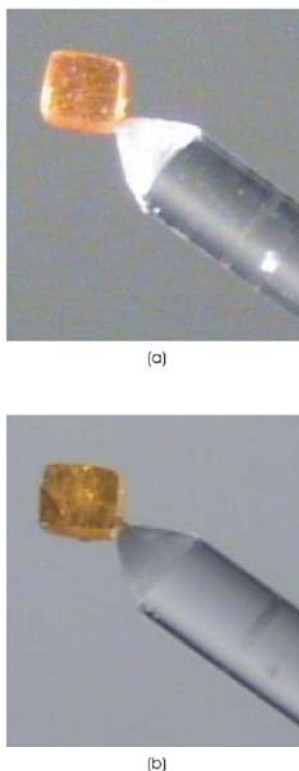
Figure 4 The crystal of [(C_4H_9NH_3)_2PbI_4] used in the diffraction experiment. (a) phase I ( -3^\circ C ) and (b) II ( -50^\circ C )
