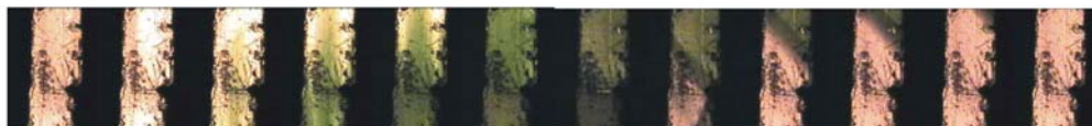
Figure 7 Optical Microscopy shows the visual evidence for the phase transitions of (C_6H_{13}NH_3)_2PbI_4 at 82^\circ C ( III to II ) and 103^\circ C ( II to I ).
