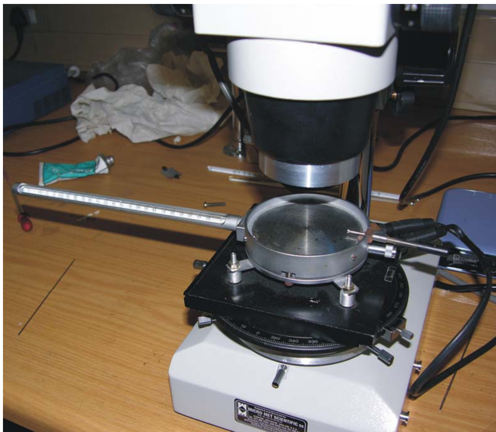
Figure 3.5: Locally modified Koffler Hot Stage.
