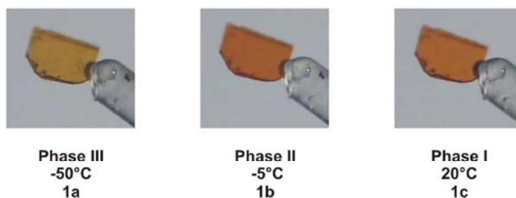
Figure 9. The colour change of a crystal of C 7 PbI. The structures of phase I ( 1c ) and II ( 1b ) were collected on this crystal. The same crystal was cooled to phase III , shown at -50°. However, a different crystal was used to collect the structure of phase III ( 1a ).
