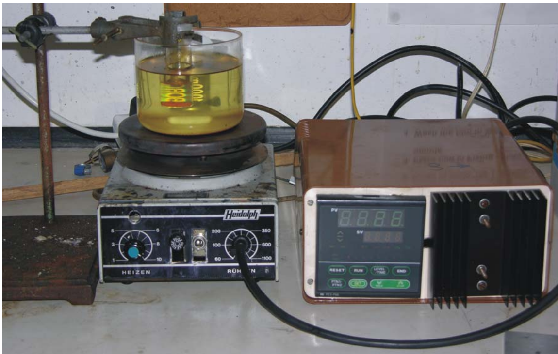
Figure 3.1: The basic experimental setup used to grow crystals of the inorganic-organic hybrids.
