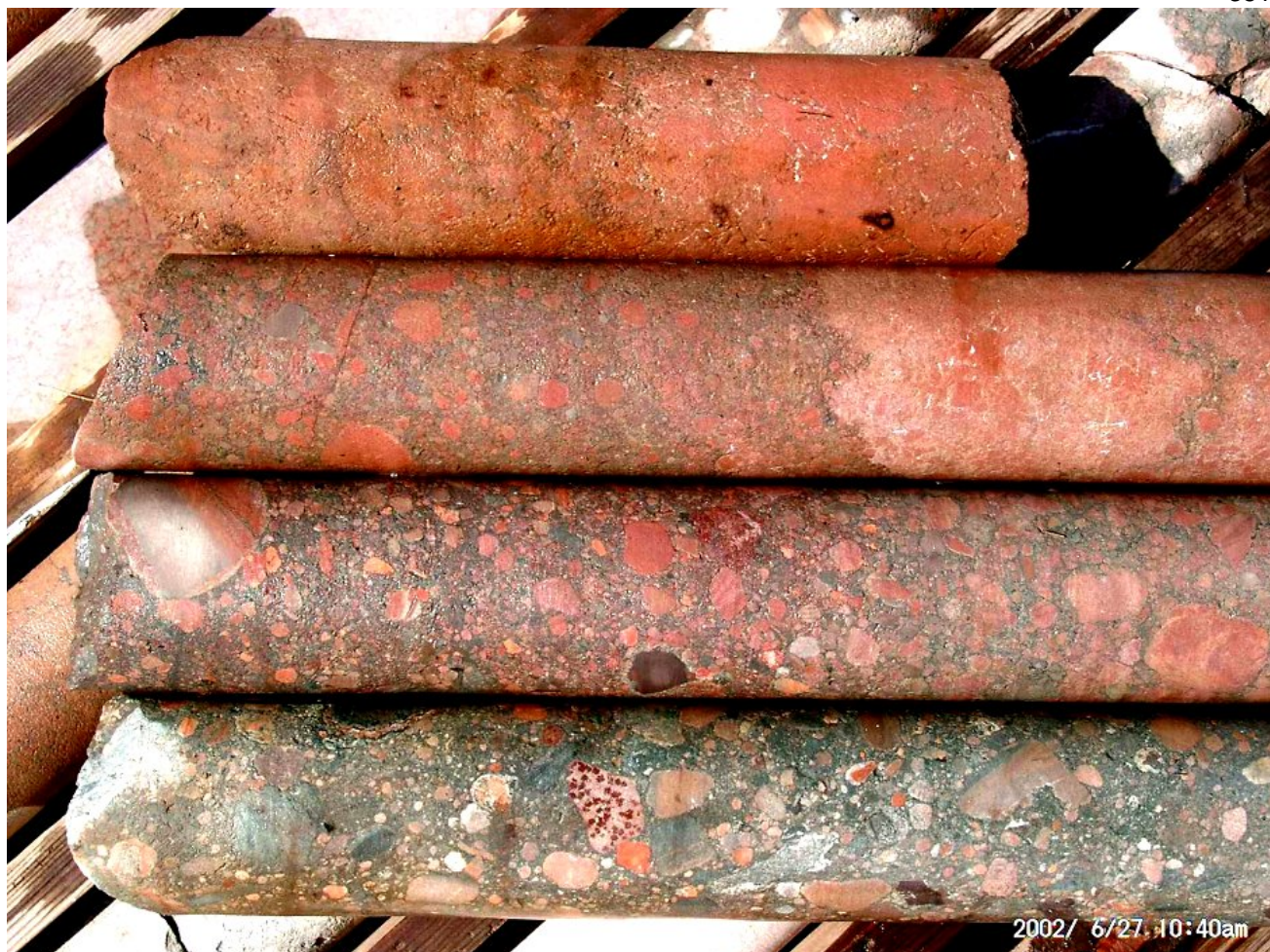
Fig 8.15 Progressive “red-rock” hydrothermal alteration in round-pebble hydrothermal breccia. The freshest rock 2 in the lower core gradually changes into an entirely deep red rock in the upper one. This is an example of hydrothermal iron oxide alteration. It can take place in almost any type of rock, obliterating previous textures and all features. Sometimes previous quartz fractures seem to be leached away and nothing is left behind except for the massive red mass full of disseminated hematite crystals. A fragment in the lower core has “hematite disease”. Note the polymictic character of the breccia and rounding of some clasts. Fragments are altered in very different ways as seen. The large fragment to the left of the second core from the bottom shows concentric hematite alteration advancing inward. Rounding of clasts will be explained in the following item. Core fragments were taken every 3 m to show variation, but a complete alteration continuum occurs in outcrop and core. From borehole MB-34, Kasempa area, Zambia. See details in text. Diameter of core is 5 cm.
