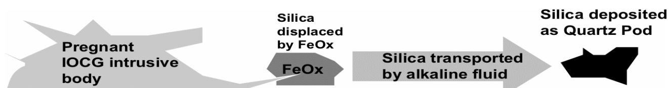
Fig 8.27 Schematic diagram to show process of quartz pod formation. Space for the emplacement of massive magnetite bodies was dissolved out from the host rocks. Silica from the dissolved minerals migrated outward from the site and later became massive quartz pods in favorable emplacement sites. All the process is carried out by warm hydrothermal fluids. This process may occur at varying scales. The radius of magnetite bodies and quartz pods may be up to a few kilometers long.
