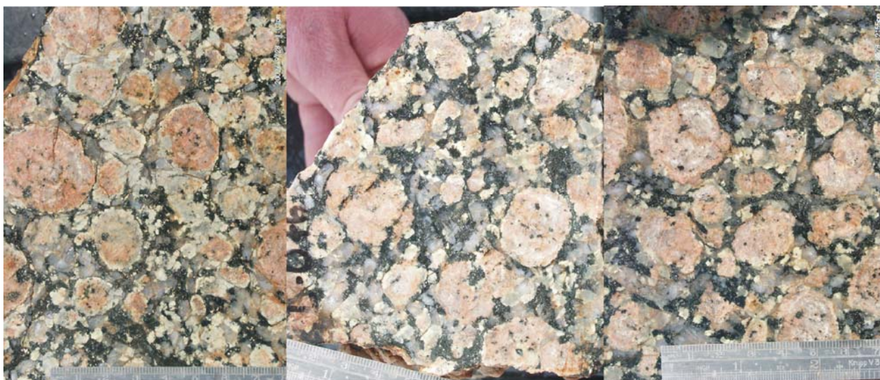
Fig 4.1.5.13 Photographs of slabs from the Muliashi Porphyry, basement to the Copperbelt, Zambia. Samples L-075 and L-076. Note the overgrowth of spherical potassium feldspar porphyroblasts. There was a previous medium-grained igneous texture that was overprinted by the macrocrysts. Most of the matrix is made of biotite. See description in text. Scales in centimeters and inches.
