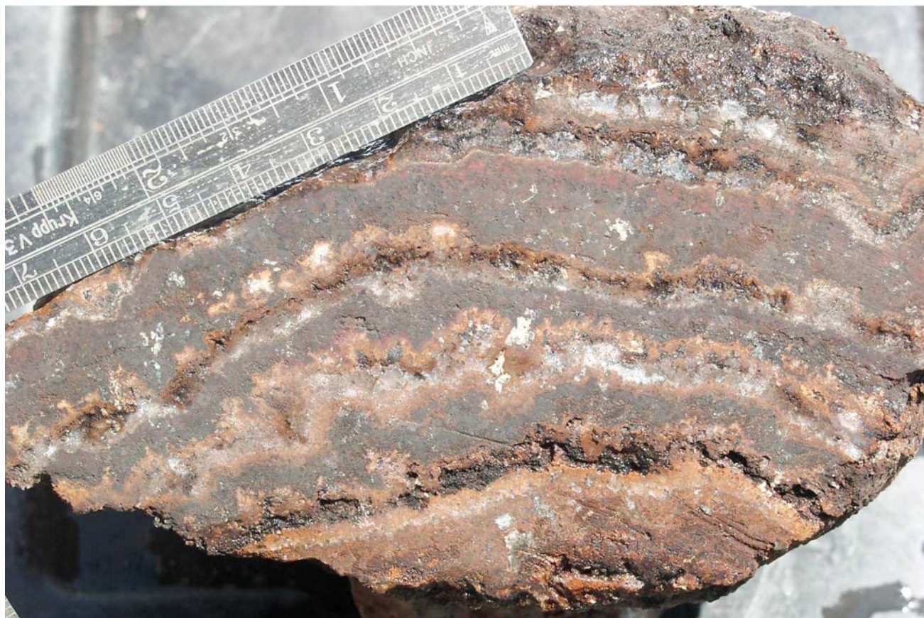
Fig 8.38 Concentric iron oxide banding around mineralized veinlets at the Dunrobin gold mine, Zambia. Host rocks in this case are Katangan carbonates, probably correlatives of the Lusaka Formation. This particular type of alteration and mineralization produces large volumes of brown, gossanous rock. When weathered, coarse free gold can be easily extracted. Parts of the main ore grade material at the mine seem to have been of this type.
