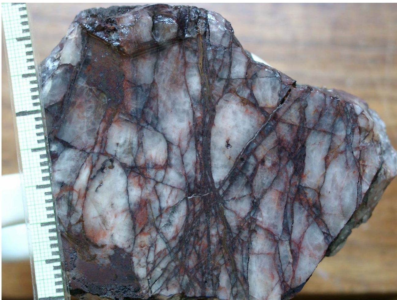
Fig 8.34 Mineralized quartz pod with magnetite and chalcopyrite. Sample L-756b from the Mesopotamie farm, Namibia. Sulfides were present in the vugs along veinlets and especially in the lower left portion of hematite,
