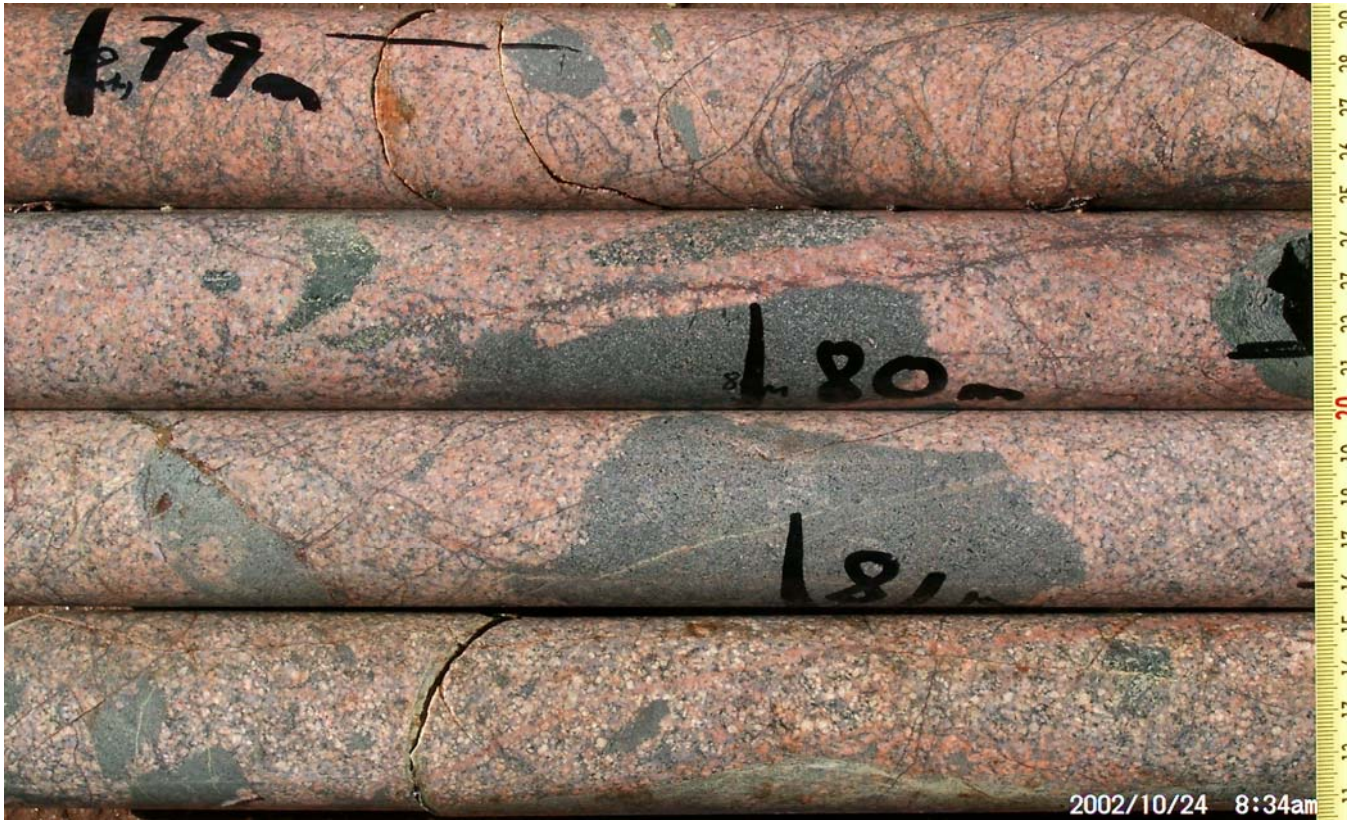
Fig 4.2.4.20. Photo 14. Core fragments from 79-82 m. At 79 m there are thin black, magnetite veinlets in stockwork. Angular fragments of black volcanic rocks and pink granitoid. Borehole OP-1, Okatjepuiko, Witvlei, Namibia.
