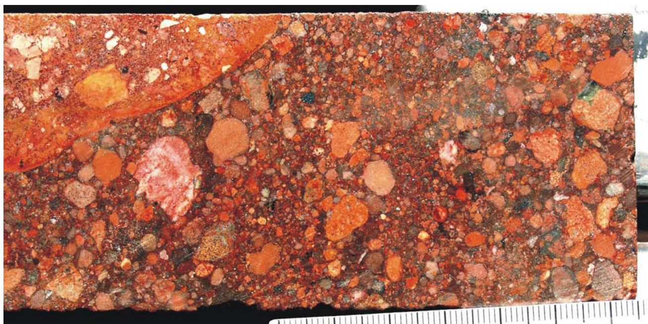
Fig 8.17 Aspect of poly-brecciated polymictic round-pebble hydrothermal breccia. The large fragment to the upper left of the photograph is composed of angular pebbles and polymictic fragments, including angular fragments of chalcopyrite and pyrite. It has been rounded itself and makes up a large clast of the new breccia. The round fragments also contain sulfide and magnetite clasts. For scale, millimetric ruler. Note that some fragments are more angular in this portion of core. From borehole MB-34, Kasempa area, Zambia. Read more details in text.
