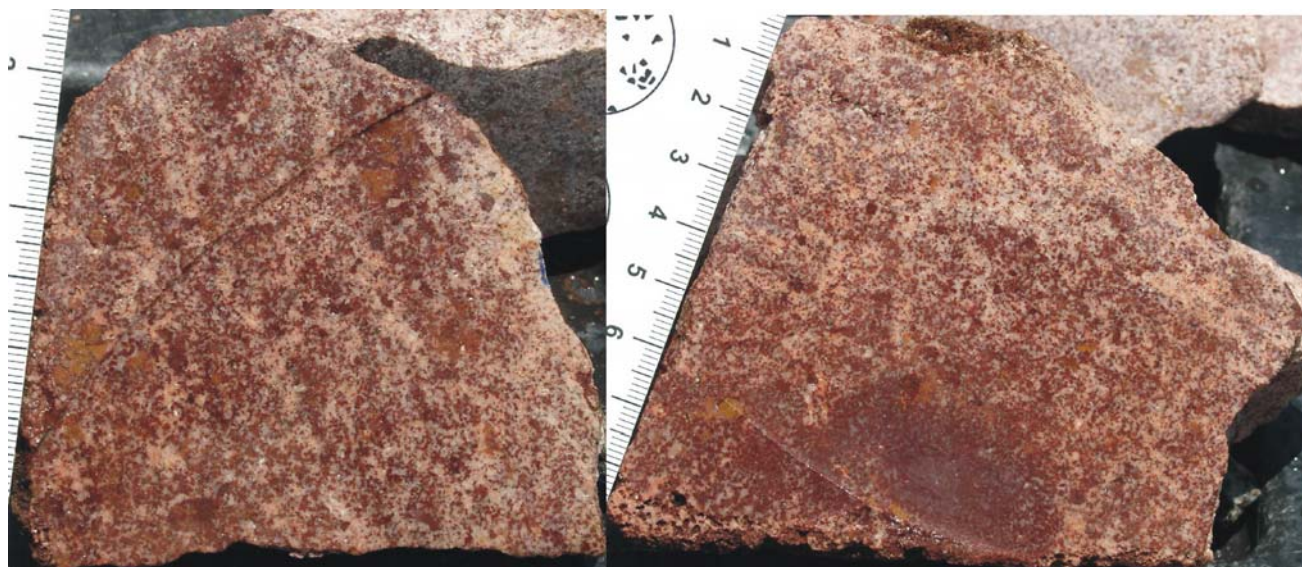
Fig 4.1.4.23 Photographs of slabs from the samples that make L-063. These rocks are essexites, and were the freshest igneous rocks available in many kilometers. Other notes in text. Scales are in millimeters.
