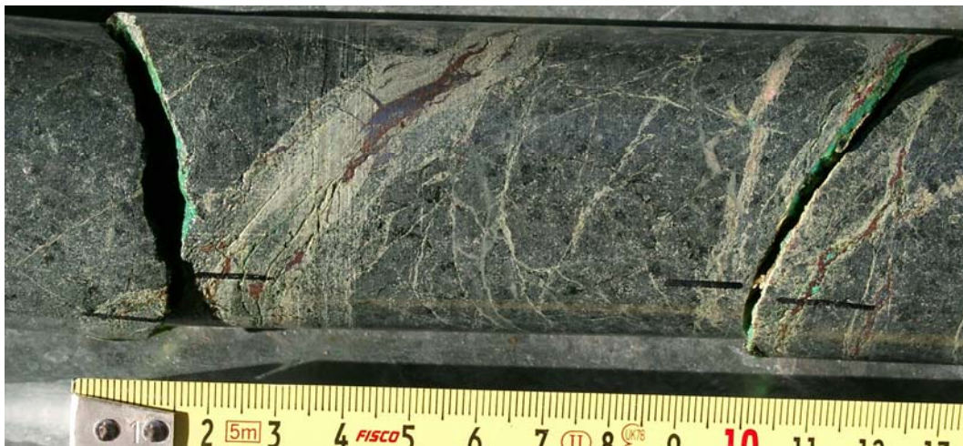
Fig 4.2.4.8. Photo 2. Enlargement with detail at 19.77 m from borehole OP-1, Okatjepuiko, Witvlei, Namibia. Note copper mineralization associated with hematite that fills part of the veinlets in a stockwork.
