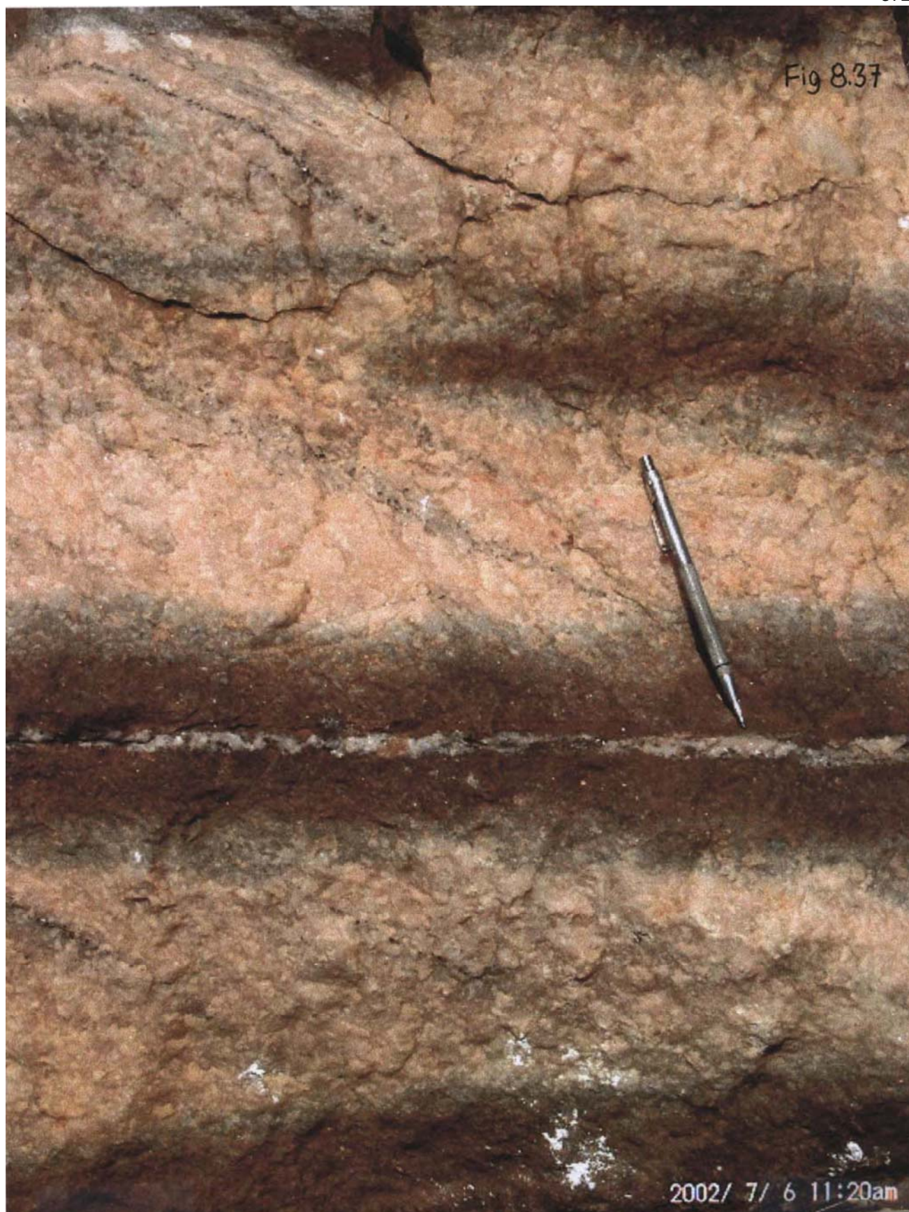
Fig 8.37 Progressive hydrothermal alteration around mineralized quartz-magnetite-sulfide veinlets at the Dunrobin gold mine, Zambia. Note steel scratcher for scale. Potassic alteration in very thin veinlets, and silicification are overprinted by later gold-bearing quartz-magnetite veinlets. Progressive hematitization of the host rock takes place away from the second generation of veinlets. Most of the host rock is heavily altered by hematitization that gives it a deep brown color. Originally the rock was a felsic granitoid. More details in text.
