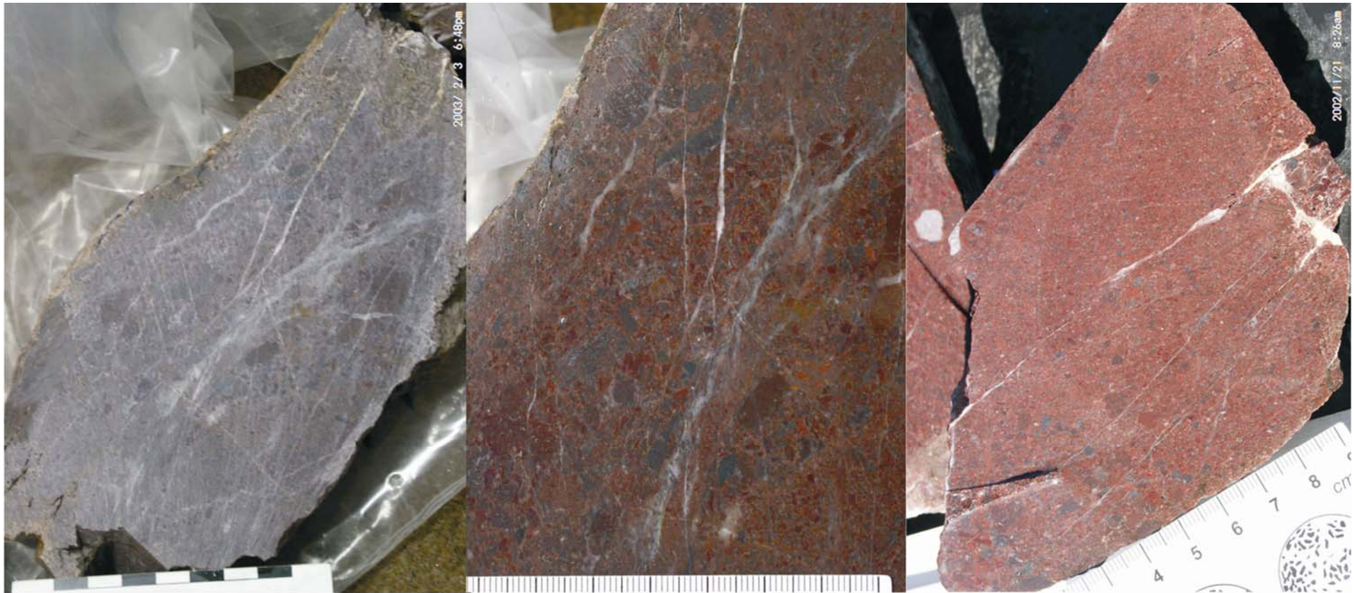
Fig 4.2.4.21. Slabs of strongly hematitized polymictic hydrothermal breccias from Samples L-644 and L-645. The left photograph was taken from a dry slab, while the other two were taken from a wet slab. Wetting enhances the contrast of the particles. The first two come from the same slab of L-644 ; the middle photo is a close-up of the first. The third photo comes from L-645 . On the second and third photos, note the angularity and variability of the clasts. The matrix has been almost completely replaced by hematite. The rock as a whole has a deep red-brown color. Abundant albite veining and strong albitization account for the rocks' induration. When hammered it produces a strong bell tinge. This type of rock forms large outcrops in the environs of the Okatjepuiko prospect. Its surface weathers to a deep brown color. In a few cases, the surface is tinted by thin layers of secondary copper carbonates, phosphates and sulphates. That takes place, even when the copper content is very low. For scale, centimeter bars on the left, and millimeters on the middle and right photos.
