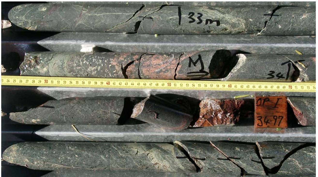
Fig 4.2.4.11. Photo 5. Beginning of hydrothermal brecciation, 33 to 34 m, borehole OP-1, Okatjepuiko, Witvlei, Namibia. Also note significant shearing in the mafic rocks.
