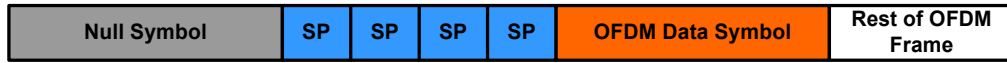
Figure 4.10: An OFDM Frame containing null and reference symbols. The reference symbol makes use of 4 synchronization patterns (SP).
