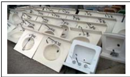
Figure 16: Reusable sinks recovered from buildings
