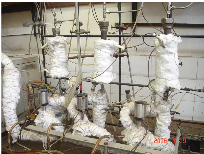
Figure 2.6: Three plug flow reactor running in parallel
