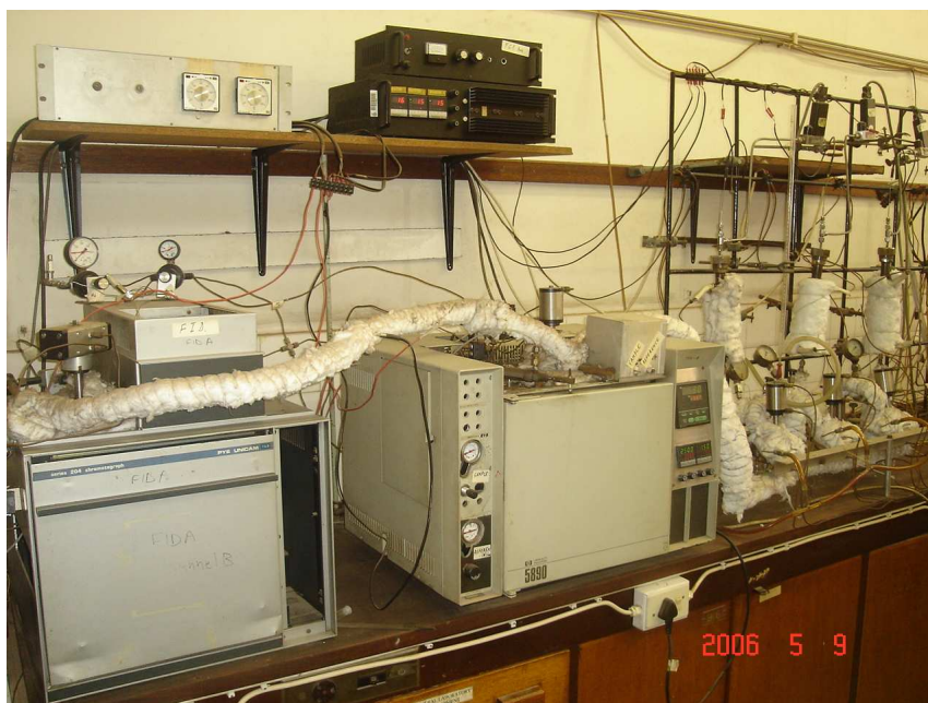
Figure 2.8: Reactor system (Reactor, two GC and temperature controllers)
