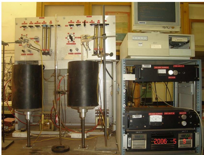
Figure 2.3: Experimental set-up for TPR measurements
