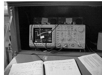
(c) Digital storage oscilloscope and fibre optic receiver enclosed in shielded box (closed during firing).
