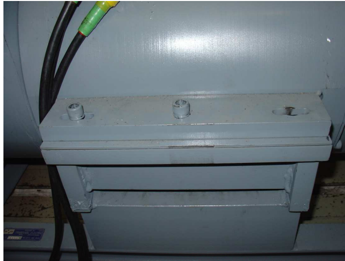
Figure 7.4: Closeup of a stator mounting bracket, showing the oblong locating holes and removable shim
