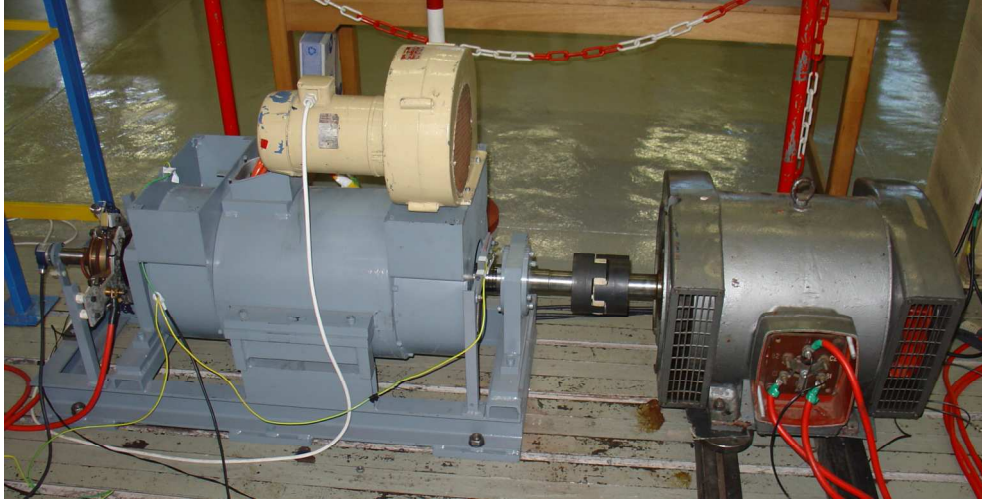
Figure 7.2: Photograph of the coupled miniature turbo-generator and 2-pole induction motor
