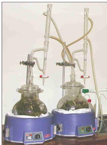
Figure 2.2: Clevenger apparatus used for distillation.
