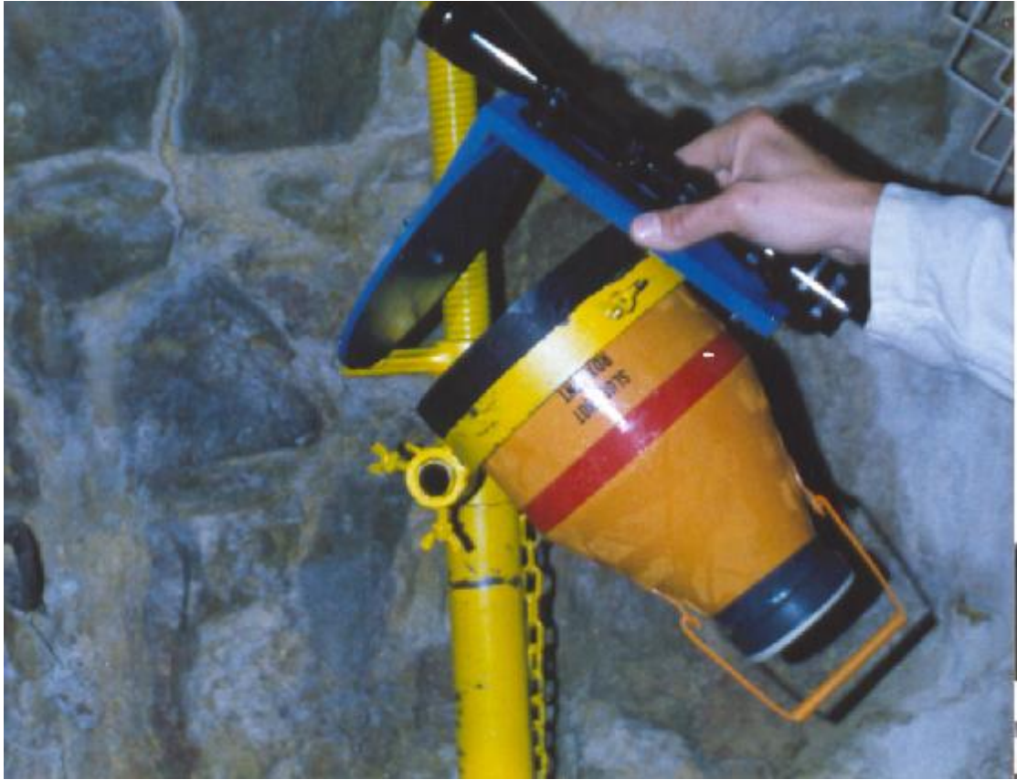
PHOTOGRAPH 2.1 SHOWING THE SLUGSHOT HANG-UP CLEARANCE CHARGE WITH IT'S ACCESSORIES UNDERGROUND
