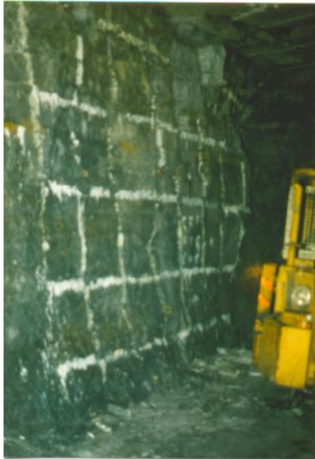
PHOTOGRAPH 9.1 SHOWING MARKED-OFF BLASTING ROUND
