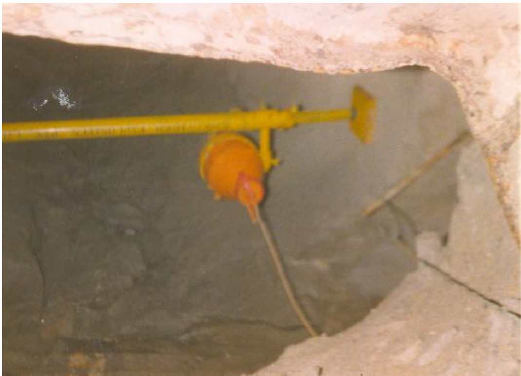
PHOTOGRAPH 2.2 SHOWING THE SLUGSHOT SET UP IN AN OREPASS WITH THE DETONATOR AND FUSE ATTACHED
