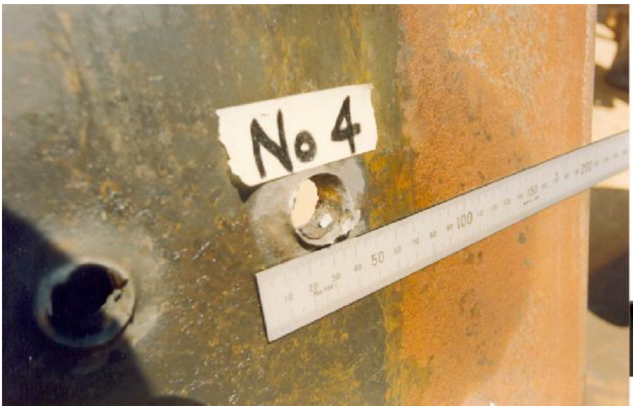
PHOTOGRAPH 7.2 SHOWING DIRECTIONAL PRIMER CHARGE POSITIONED ON A WITNESS PLATE
