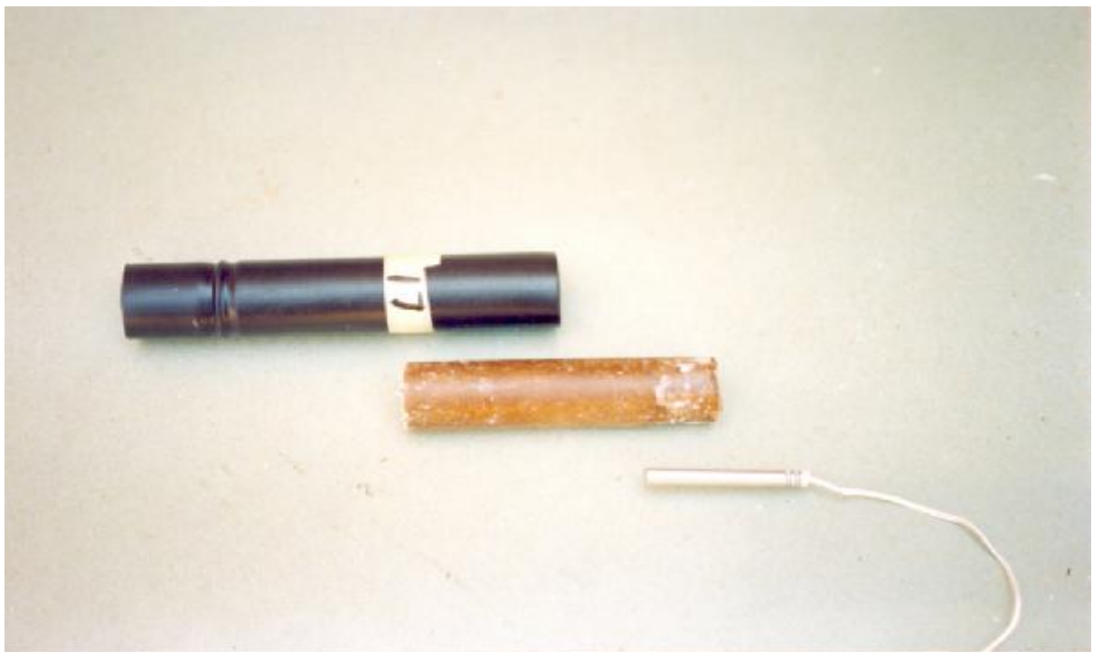
PHOTOGRAPH 7.1 SHOWING DIRECTIONAL PRIMER CHARGE DETONATION CHAIN
