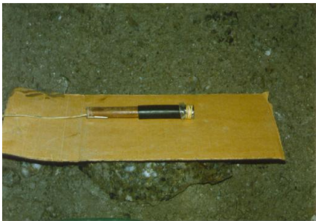
PHOTOGRAPH 9.2 SHOWING 32 MM DIAMETER DIRECTIONAL PRIMER CHARGE CARTRIDGE WITH PLASTIC WRAPPER AND ELASTIC BAND COVERING OF OPEN END TO PREVENT INGRESS OF DRILL CHIPPINGS
