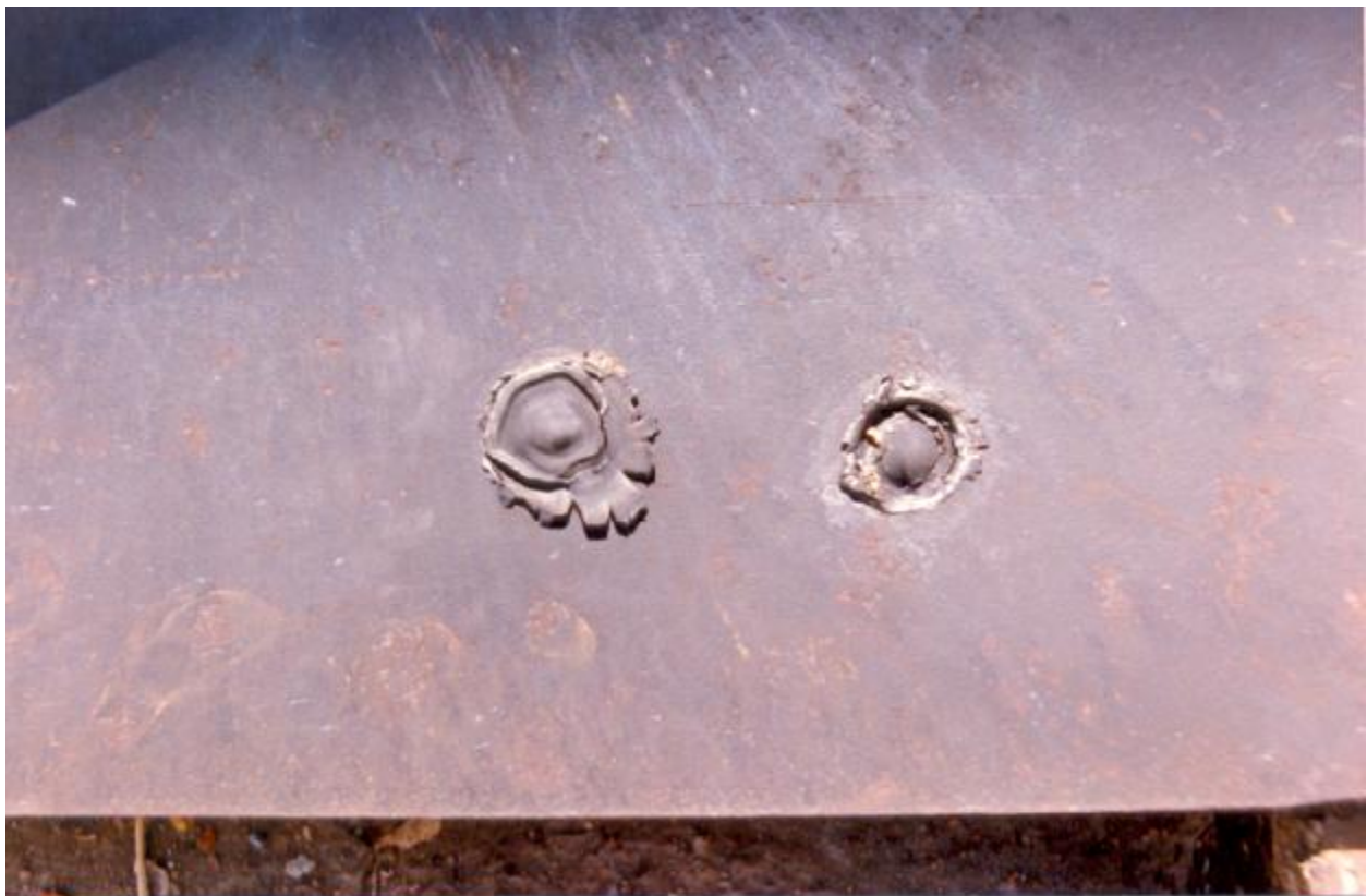
PHOTOGRAPH 7.6 SHOWING TWO SLUGS EMBEDDED IN WITNESS PLATES
