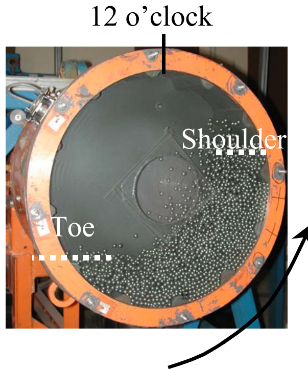
Figure 5.2 Load orientation profile description
