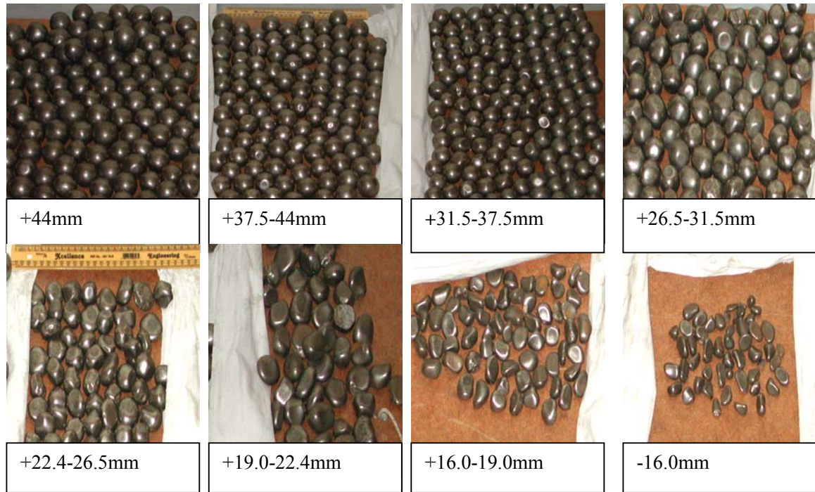
Figure 4.6 Characteristic features of balls inside ball mill
