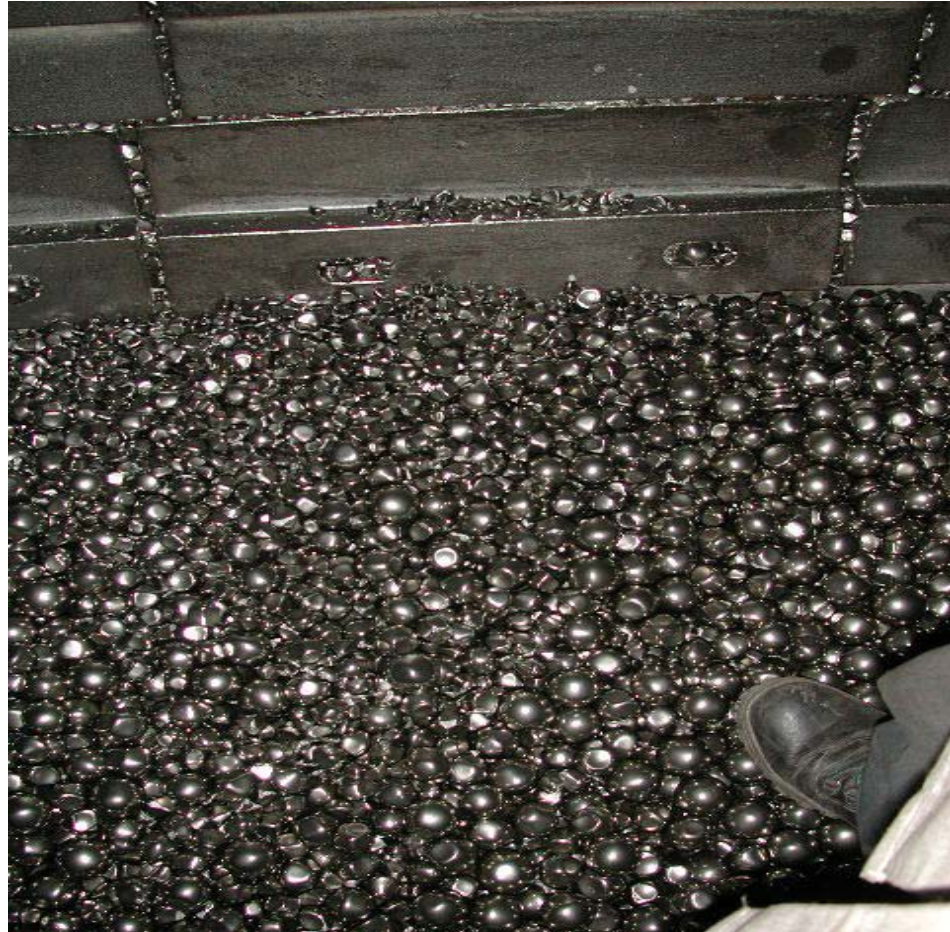
Figure 1.1 Characteristic shapes of balls inside a ball mill
