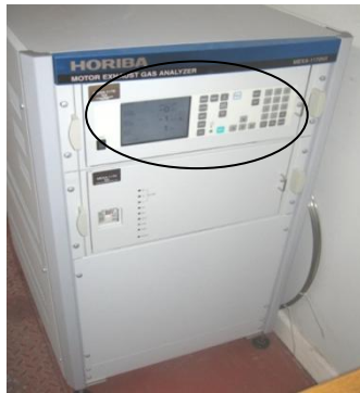
Fig 4.9: MEXA-1170 Nx. [Tamaldin, 2010] The MEXA and the EXSA share some of the gases, therefore the gas lines exiting the regulators inside the test cell were teed off to fit both analysers. The control panel (circled) was used to operate the MEXA during the experiments as the MEXA could not be controlled via the Texcel v12.
