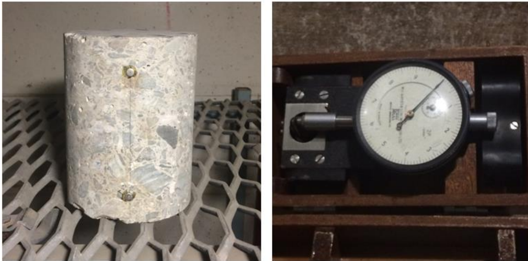
Figure 3-3 – Concrete core with DEMEC studs (left) and strain gauge (right)
