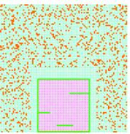
Figure 9. Convection Heat Model View. Air cells (Light Green and Light Red), Wall (Green), Heat-Source (Dark Red) and Insulation (Orange).
