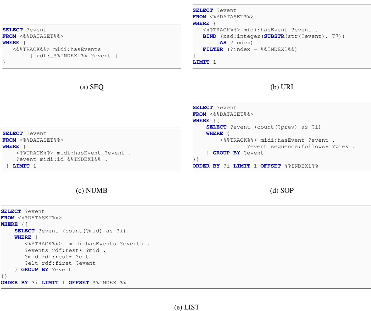
Fig. 6. Queries for the GET operation. The operation is supposed to return the entity at a given position in the list. In the minimal form, the operation returns the URI of the entity. It can be seen how each modelling solution requires a SPARQL query using different language operators. In some cases, it was impossible to avoid subqueries in order to compute the position of each item in the list and compare it with the required index.
