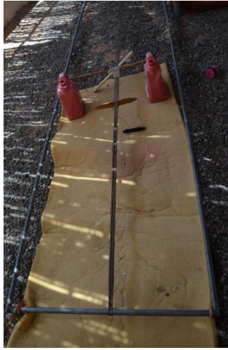
Figure 4-67 Siim tool (two pieces of woods sloped on two long steel tubes, stood on plastic cans) (Photographed by Amal Al-Ismaili, North Sharqiyah, Oman, 2016)
