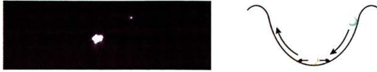
Figure 3.4. A single trapped particle residing in a potential well created by two aligned counter-propagating beams.
