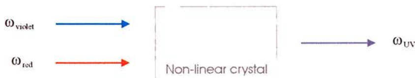
Figure 6.2. The photon model represents frequency conversion of two fundamental wavelengths interacting with the non-linear crystal into a higher frequency.
