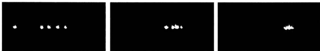
Figure 3.7. A fifth 2.3\ \mu\text{m} particle guides into an array of four spheres along the right propagating beam. This creates an unbalance to the forces that can cause instability to particles causing the collapse of an array. The series of images shown here demonstrates the array collapsing into a central clump, which remains in the potential well.
