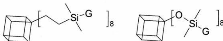
Figure 8.1: Metal Organic Framework precursors synthesised from vinyl POSS and TMA silicate illustrating the more rigid structure produced by the use of TMA silicate. G is a generic substituent
