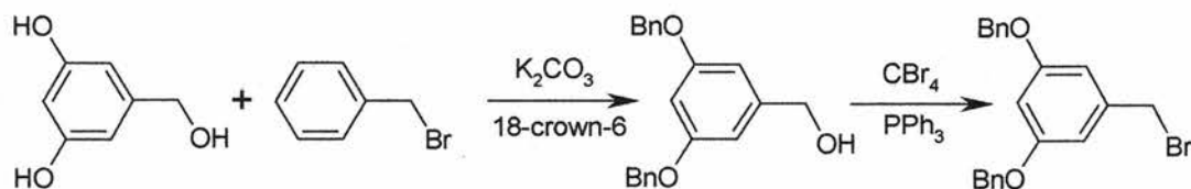
Figure 1.18: Synthesis of Fréchet type wedges, poly (benzyl ether).
