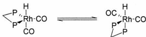
Figure 5.4: Diequatorial (ee) to equatorial-apical (ea) binding modes of bis-diphenylphosphine complex.
