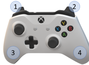
Fig. 3. Microsoft Xbox One wireless controller, showing position of embedded trigger (1,2) and palm (3,4) ERM motors, and button layout.
