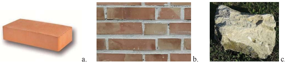
Figure 7: a. Used materials for wall construction: Solid bricks (240 x 120 x 55 mm); b. Bonding pattern, c. Ashlar calcareous stone.
