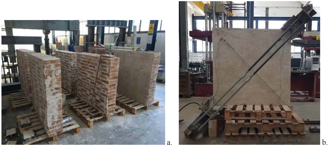
Figure 2: Realization of full-scale shear walls: a. Solid bricks test specimens, b. shear test setup.
