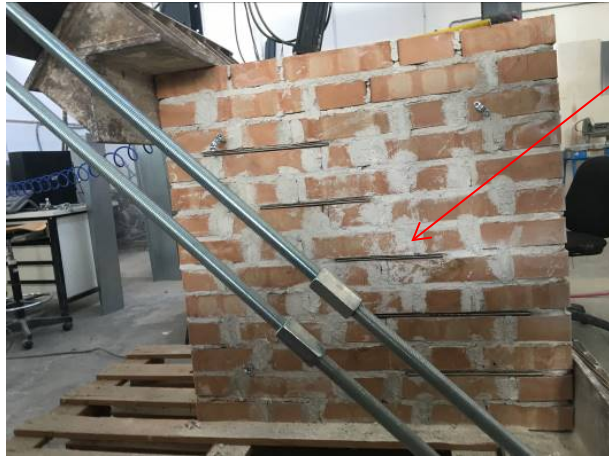
Figure 17: A repaired wall panel using titanium rods for crack stitching.
