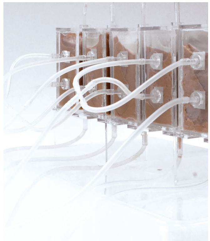
2 Prototype 2, casting vessel showing connection between the suspended mold and the bioreactor.
