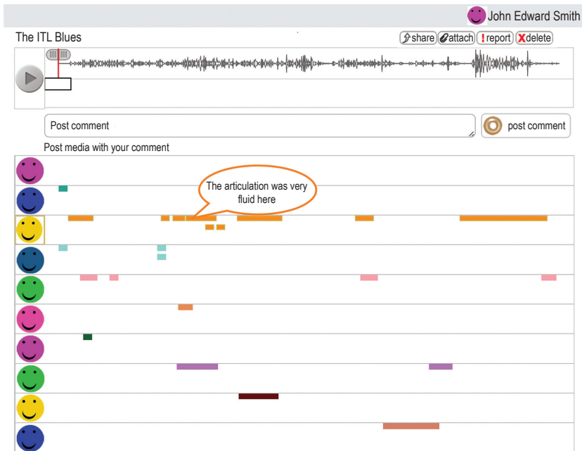
Figure 14.1 Screen shot of the MusicCircle system, showing an audio recording being annotated. At the top is the waveform, then below is the social timeline showing the annotations of various members of the community. This audio recording and the associated dataset is available at http://zenodo.org/record/46232 (accessed Feb. 11, 2019).
