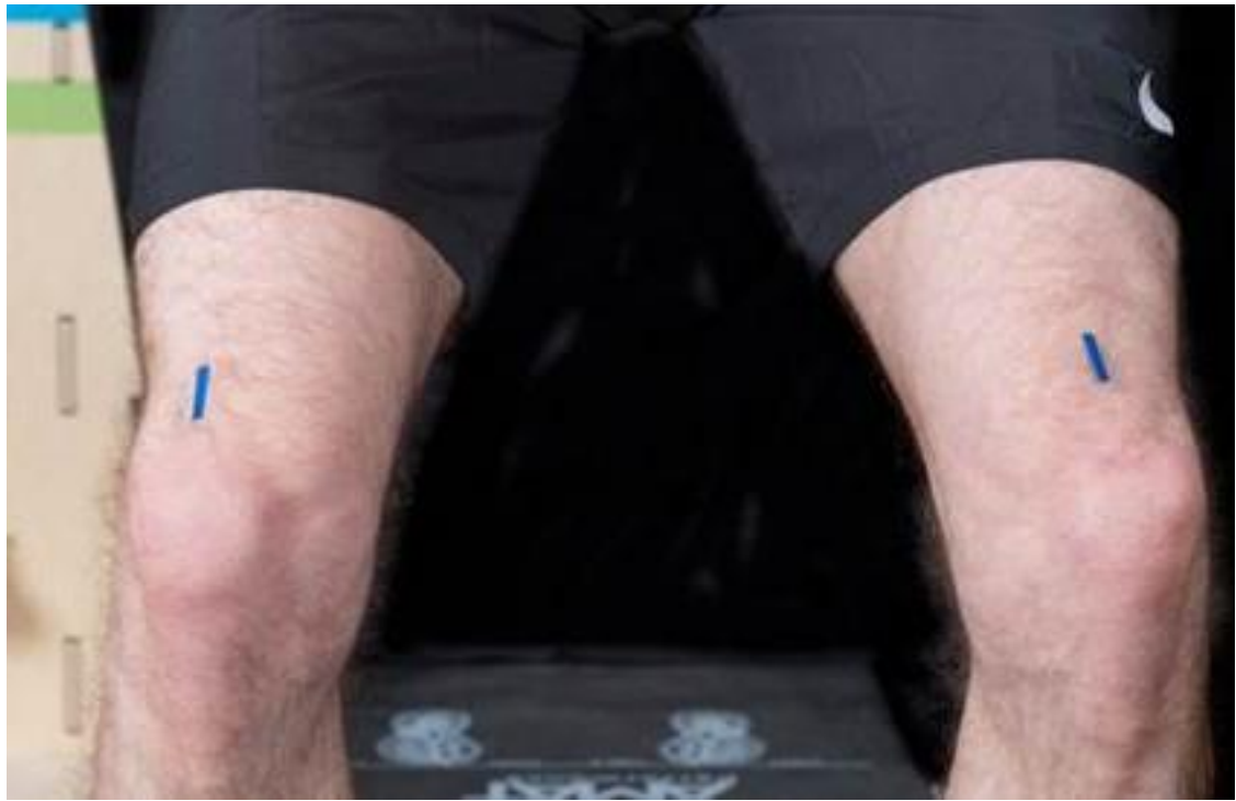
Figure 3.14. Retroreflective knee markers placed on top of each patella.
