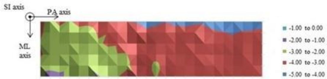
Figure 3.17. Surface area plot prior to inclusion of the second calibration algorithm. The different colours in the figure represent the difference in centimetres between the real position and the position obtained by the Kinect TM in the posterior-anterior axis. The legend displays the difference in centimetres every colour represents. The measure unit of the axis and the legend is centimetres.
