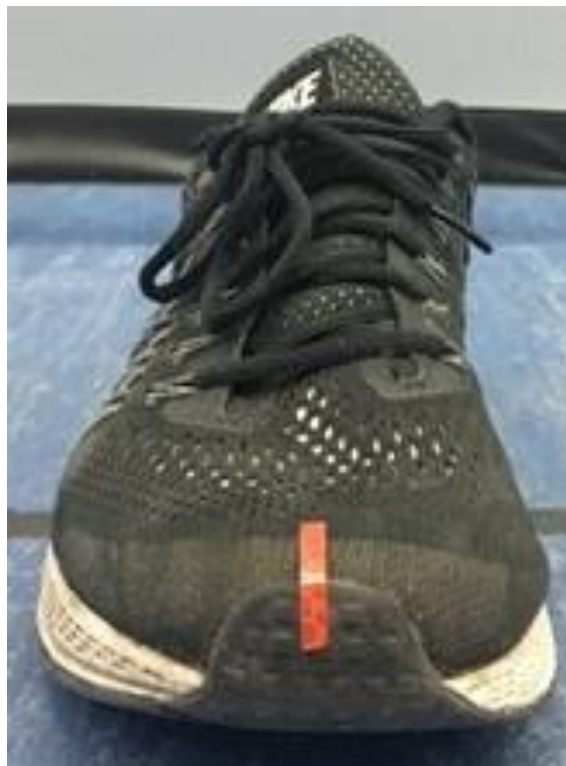
Figure 3.9. A trainer with the original retroreflective infrared marker (red string) attached to it. The idea for such a marker was based on MacPherson et al. (2016).
