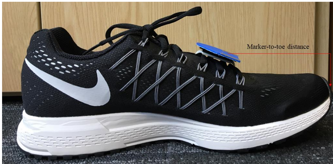
Figure 5.1. A shoe with the foot marker attached to the lace. The Marker-to-Toe distance is displayed by the red arrow and is the distance in the posterior-anterior axis from the centre of the foot marker to the toe of the shoe.
