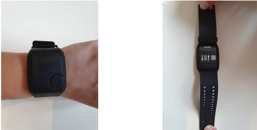
FIGURE 5.2: Empatica E4 wristband which was used to gather EDA and HRV. The picture shows the placement of the wristband (left) and the location of the PPG sensor (right).
