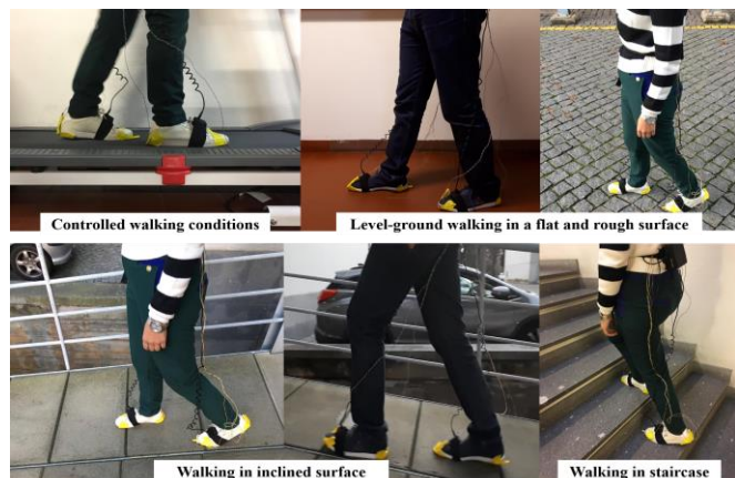
Fig. 6. Validation of the gait event detection system under controlled and real-life walking conditions (flat and rough level-ground, inclined surfaces and staircases). The users wore two units of InertialLAB (instead of the foot) and two FSRs attached to heel and toe by a yellow rubber strap.
