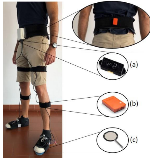
Figure 2. Wearable Motion LAB sensor placement. (a) Infrared laser sensor. (b) Xsens IMU sensor. (c) FSR ground reaction force sensor
