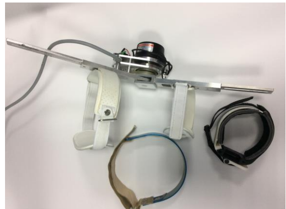
Figure 2 – Orthosis with straps used to fix the device to human's limb.
