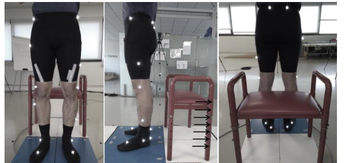
Figure 2. Photograph of the markers placed on the subject and the seat used in the experimental test.
