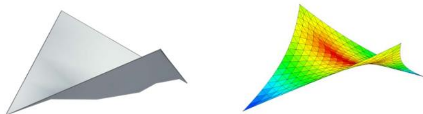
Figure 58 – Starting geometry (left), and the structure analysed under load applied (right). (colours indicate the wrap stress). Adapted from Henrysson (2012).
