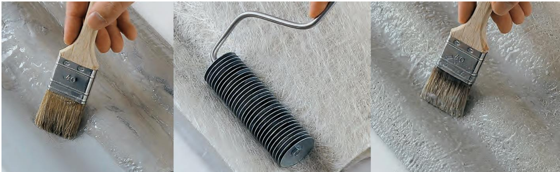
Figure 30 - Process of manual lamination of GFRP. (Knippers, Cremers et al. 2011)
