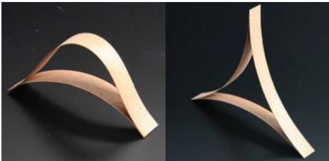
Figure 3 - Basic bending-active components. (Lienhard 2014)
