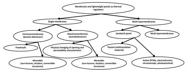
fig.01 - Classification of membranes and lightweight panels as thermal regulating elements [Mendonça, 1997]
