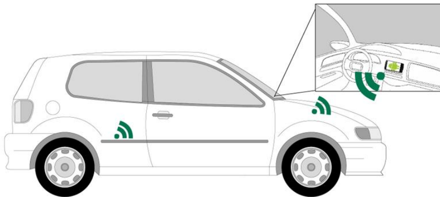
Figure 2. Placement of the nodes of the BLE network inside of the car.
