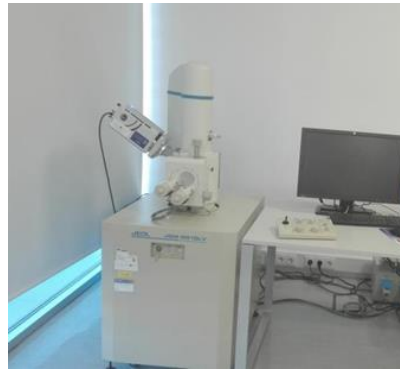
Figure 4.12: Field Emission Gun Scanning Electron Microscope (FEGSEM) with an Energy Dispersive Spectroscopy (EDS)
