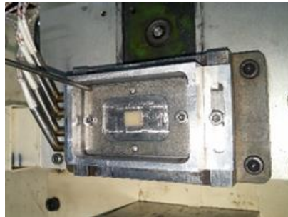
Figure 4.6: Detail of the mounting plate and one of the samples of the composite material
