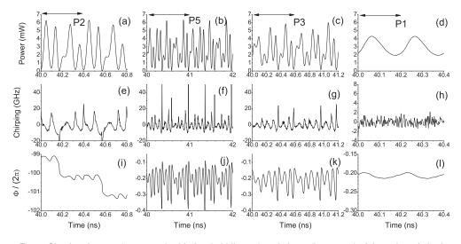
Fig. 9. Simulated power (upper row), chirping (middle row) and phase (lower row) of the gain-switched SL laser ( $I_{bias}=30$  mA,  $f_R=5$  GHz, and  $V_{RF}=0.5$  V) with optical injection at detuning  $\Delta \nu_i=4$  GHz and different values of injected power  $P_i$ , (a), (e), (i) 250  $\mu$ W, (b), (f), (j) 338  $\mu$ W, (c), (g), (k) 416  $\mu$ W, (d), (h), (i) 2300  $\mu$ W. In this figure  $\kappa_c=1.5\times10^{11}s^{-1}$ .
