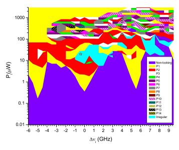
Fig. 7. Experimental values of the injected power as a function of the frequency detuning at which different dynamical regimes are observed for  $l_{bias}=30$  mA,  $f_R=5$  GHz, and  $V_{RF}=0.5$  V. White stars correspond to cases illustrated in Figs. 8 and 10.
