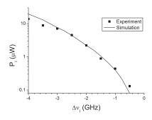
Fig. 5. Experimental (squares) and simulated (solid line) injected power necessary to get P1 dynamical regime as a function of the frequency detuning. In this figure  $l_{bias} = 30$  mA,  $f_R = 5$  GHz, and  $V_{RF} = 1$  V.
