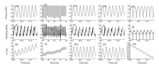
Fig. 4. Simulated power (upper row), frequency chirping (middle row) and optical phase (lower row) of the gain-switched SL ( $l_{bias} = 30$  mA,  $f_R = 5$  GHz, and  $V_{RF} = 1$  V) with optical injection at detuning  $\Delta v_i = -2$  GHz and different values of injected power  $P_i$ , (a), (f), (k) 41 nW, (b), (g), (l) 1.9  $\mu$ W, (c), (h), (m) 3.67  $\mu$ W, (d), (i), (n) 14  $\mu$ W, (e), (j), (o) 415.4  $\mu$ W.
