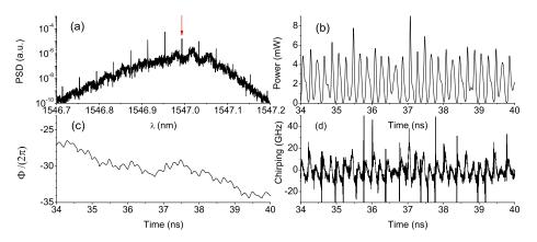
Fig. 10. Simulated (a) optical spectrum, and time traces of (b) power, (c) optical phase, and (d) frequency chirping at  $l_{bias} = 30$  mA,  $f_R = 5$  GHz,  $V_{RF} = 0.5$  V,  $\Delta v_i = -0.4$  GHz, and  $P_i = 20$   $\mu W$ . In this figure  $\kappa_c = 1.5 \times 10^{11} \, s^{-1}$ . The wavelength of the optical injection is indicated with an arrow.
