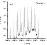
Fig. 2. Experimental (a) and simulated (b) optical spectra (PSD: Power Spectral Density) of the gain-switched laser ( $l_{bias}$  =30 mA,  $t_R$  = 5 GHz, and  $v_{RF}$  = 1 V) without optical injection .
