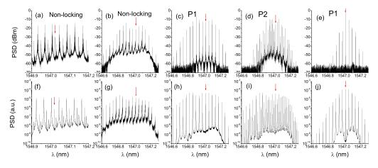
Fig. 3. Experimental (upper row) and simulated (lower row) optical spectra of the gain-switched laser ( $l_{bias} = 30$  mA,  $f_R = 5$  GHz, and  $V_{RF} = 1$  V) with optical injection at detuning  $\Delta \nu_i = -2$  GHz and different values of injected power  $P_i$ , (a), (f) 41 nW, (b), (g) 1.9  $\mu$ W, (c), (h) 3.67  $\mu$ W, (d), (i) 14  $\mu$ W, and (e), (j) 415.4  $\mu$ W. The injection frequency is indicated with an arrow.
