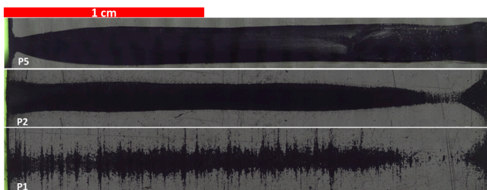
Figure 6. Stacked microscopic images of PA joint area after failure (dark areas), illustrating effect of laser-ablation parameters on joint quality.
