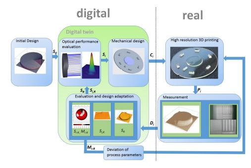
Figure 2. Simplified visual illustration of digital twin and process flow.
