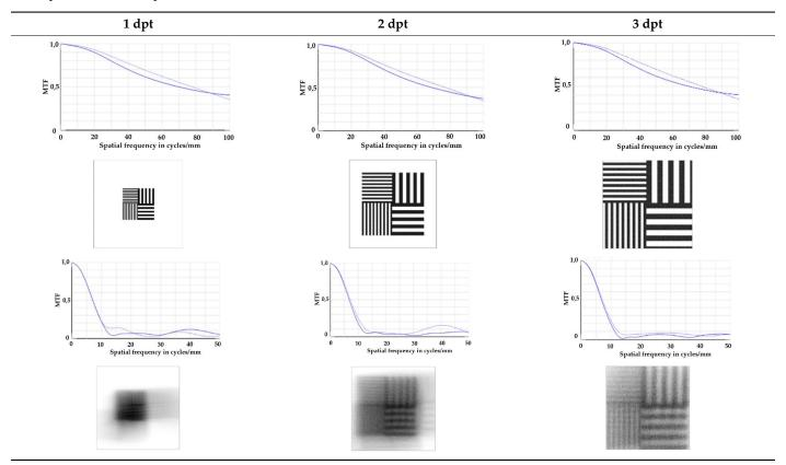
**Table 1.** The modulation transfer function (MTF) and geometric image analysis of three different adjustments of the rotation optics (1, 2, and 3 dpt) for the nominal surface (first row) and the measured data (second row).
