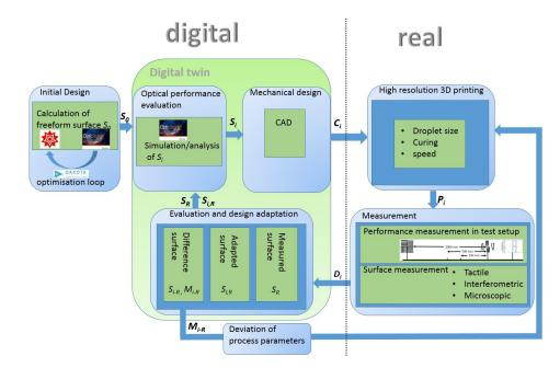
Figure 1. Digital twin and process flow.
