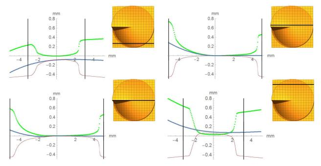
**Figure 7.** Measured profile (red), nominal profile (blue), and difference profile (green) inside the nominal aperture (solid black and perpendicular lines). Insets: position of the respective profile on the surface.
