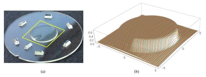
parallel to the surface discontinuity of the rotation optics. Figure 5b shows a superelevated 3D-plot of the 210 measurement profiles, each containing 5250 data points.
