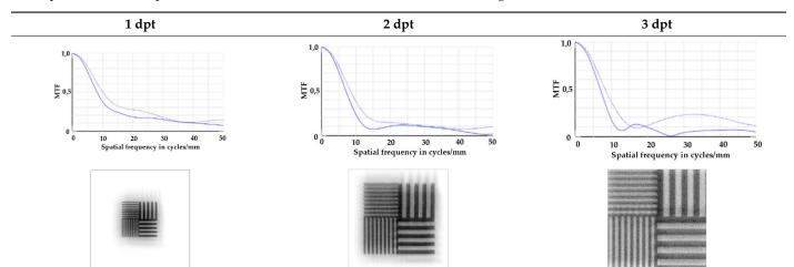
**Table 2.** Modulation transfer function (MTF) and geometric image analysis of three different adjustments of the rotation optics (1, 2, and 3 dpt) for the nominal surface constraint with a manufacturing tolerance of  $\pm 10 \,\mu$ m.
