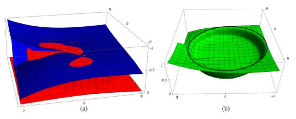
**Figure 6.** (a) Overlay of nominal surface (blue) and measured surface (red); (b) difference surface. The black circle indicates the nominal aperture.
