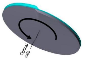
**Figure 4.** Rotation optics, consisting of two lens bodies with surfaces of azimuthal curvature dependence arranged coaxially to the optical axis and their plane surfaces facing each other [27].
