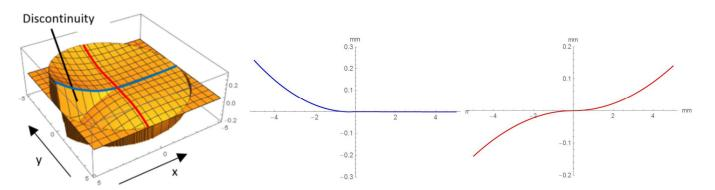
**Figure 3.** Left: Superelevated geometry of a lens surface with lines of intersection parallel to the x-axis (blue) and parallel to the y-axis (red). Middle: Profile parallel to x-axis along the blue intersection path. For positive abscissae, the ordinates are zero and the curve directly superimposes the x-axis. Right: Profile parallel to y-axis along the red intersection path [21].
