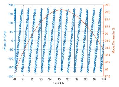
Fig. 5 Complex  $HE_{11}$  mode amplitude at the mode converter output. Phase response (blue circles). Squared absolute value (brown curve)
