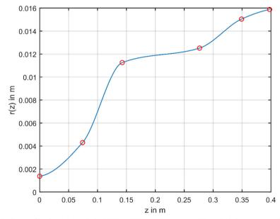
Fig. 4 Radius profile along the optimized  $TE_{11} \mapsto HE_{11}$  mode converter. The red circles represent the single chromosomes, used for optimization
