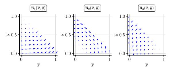
**Figure 2.4:** Vector basis functions  $\overline{\mathbf{n}}_1(\overline{x}, \overline{y})$ ,  $\overline{\mathbf{n}}_2(\overline{x}, \overline{y})$ , and  $\overline{\mathbf{n}}_3(\overline{x}, \overline{y})$  of degree n = 1 used to expand the solution of the electric field in a reference isosceles right triangle  $\mathcal{T}_0$ . The vector functions are defined by Eqns. (2.79)-(2.81).
