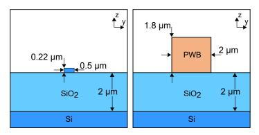
**Figure 5.9:** Cross sections of the silicon waveguide, left, and the photonic wire bond waveguide, right. Both elements are placed on top of a layered substrate composed of silica (SiO<sub>2</sub>) ad silicon (Si) and are embedded into a material with a permittivity of  $\epsilon_{\text{cladding}}$  at the operating wavelength of 1.55 µm.
