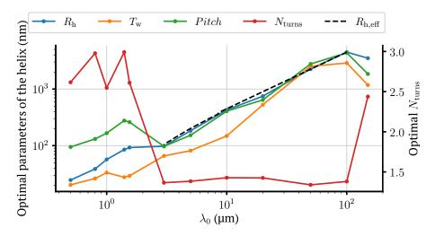
**Figure 5.3:** Design parameters of the optimal helices obtained in the optimization runs made for different design wavelengths. The design parameters are the radius of the helix spin,  $R_h$ , the thickness of the helix wire,  $T_w$ , the pitch of the helix, *Pitch*, and the number of turns of the helix,  $N_{turns}$ . The schematic of Fig. 5.1 shows the meaning of the different parameters in more detail.
