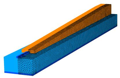
**Figure 5.12:** FEM discretization of the waveguide coupler. Due to the symmetry of the structure, only half of the device needs to be discretized for the finite element method simulation.
