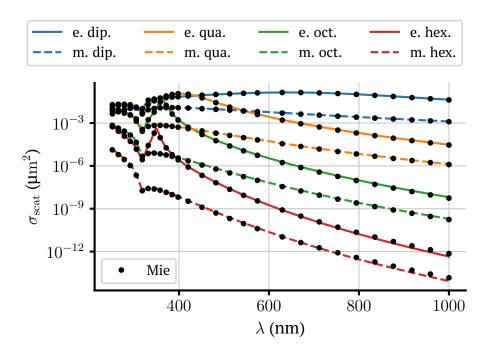
**Figure 4.3:** Multipole decomposition of the field scattered by a silver sphere illuminated by a plane wave. The wave vector of the plane wave is oriented in the -z-direction. Its electric field is linearly polarized in the *x*-direction with an amplitude of 1 V/m. The sphere has a radius of 112.5 nm and its permittivity at each wavelength is interpolated from a database [230].
