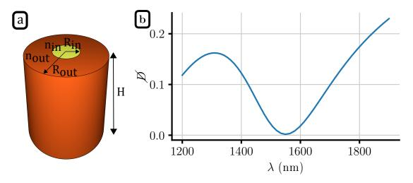
**Figure 4.10: a.** Sketch of the considered core-shell disk. Its geometrical parameters are  $R_{\rm in} = 111$  nm,  $R_{\rm out} = 237$  nm, and H = 431 nm. The core and the shell are made of materials with nondispersive permittivities of  $\epsilon_{\rm in} = 10.63$  and  $\epsilon_{\rm out} = 5.3$ . **b.** Wavelength dependency of the duality breaking,  $\mathcal{D}$ , of the optimal core-shell disk around the central wavelength of 1.55 µm.
