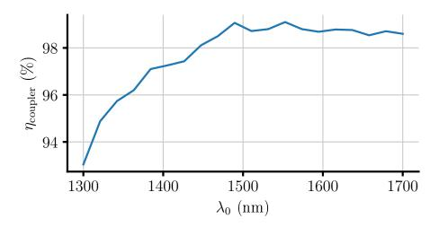
**Figure 5.16:** Coupling efficiency of the optimal adiabatic taper as a function of the wavelength of the illuminating waveguide mode. The parameters of the optimal coupler are shown in the caption of Fig. 5.14.
