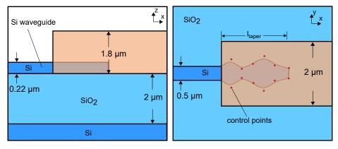
**Figure 5.18:** Schematic of the freeform waveguide edge coupler. The shape of the coupler is described by a NURBS curve, defined by a series of control points. The control points, shown in the schematic as red dots, are equispaced in the x-direction and they are allowed to move only in the y-direction.
