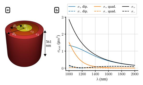
**Figure 4.9:** Scattering cross section of a core-multi-shell disk decomposed into the fields scattered with both helicities. The disk is illuminated with a right circularly polarized plane wave with an amplitude of 1 V/m. The wave vector of the plane wave is oriented in the +*z*-direction. The object is composed of three concentric disks with the same height, 361 nm, and radii 157.9 nm, 284.8 nm, and 375 nm. Their corresponding permittivities are 3.61, 11.16, and 4.84, respectively.
