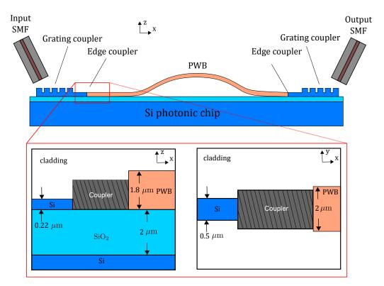
**Figure 5.8:** Schematic of the architecture for an optical inter-chip communication system.
