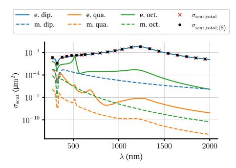
**Figure 4.5:** Cross section of a nanorod calculated using two different methods: the multipole expansion and the integral of the power flux of the scattered field. The nanorod is a silver ellipsoid with a semi-major axis of 225 nm and semi-minor axis of 37.5 nm. The major axis is oriented along the *x*-direction. The nanorod is illuminated with a plane wave with the wave vector parallel to the -z-axis and the electric field linearly polarized in the *x*-direction.
