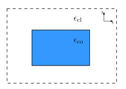
**Figure 2.2:** Sketch of a dielectric rectangular waveguide. The waveguide has a rectangular core with permittivity  $\epsilon_{co}$ . The core is surrounded by the cladding, which extends till infinity and has a permittivity  $\epsilon_{cl}$ . The geometry of the waveguide is invariant along *z*-direction.
