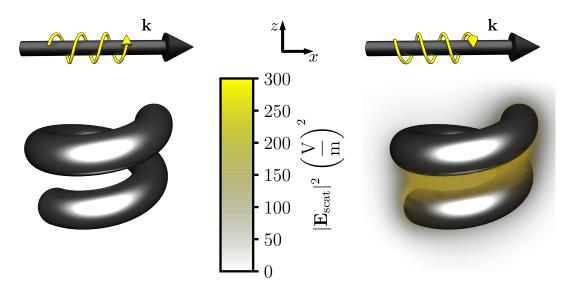
**Figure 5.6:** Intensity of the field scattered by a helix as a function of the handedness of the illuminating circularly polarized plane wave. The results are shown for the optimal helix obtained from the optimization run at  $\lambda_0 = 3\mu m$ . The illumination direction relative to the helix is indicated in the top of the figure.
