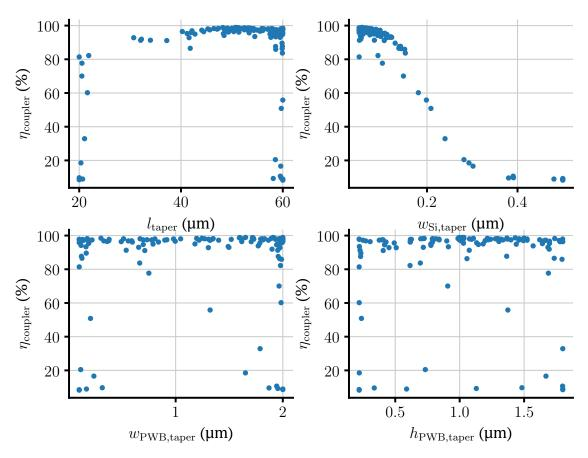
**Figure 5.13:** Coupling efficiencies of the different designs evaluated during the optimization process of the linear taper edge coupler. Each figure show the projection of the coupling efficiency values over the different parameters of the design space. The parameters are defined in the schematic of Fig. 5.11.
