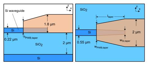
**Figure 5.11:** Schematic of the parametric waveguide coupler. The coupler is parametrized by its length,  $l_{taper}$ , the height,  $h_{PWB,taper}$ , and width,  $w_{PWB,taper}$ , of the photonic wire bond at its opening facet and by the width of the silicon core of the taper at its edge,  $w_{Si,taper}$ .
