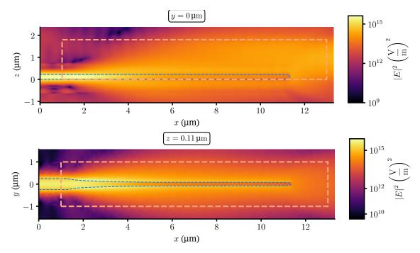
**Figure 5.20:** Intensity field distribution along the optimal freeform coupler obtained for a coupler length of 10 µm. The coupler achieves a performance of  $\eta_{\text{coupler}} = 91\%$ .
