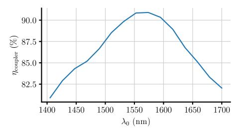
**Figure 5.21:** Dependency of the coupling efficiency,  $\eta_{\text{coupler}}$ , for the optimal freeform edge coupler shown in Fig. 5.20 with respect to the excitation wavelength. The wavelength values are those corresponding to the wavelength in free space. The coupler has been optimized for a wavelength of 1.55 µm, which corresponds with the position of the peak for the coupling efficiency.
