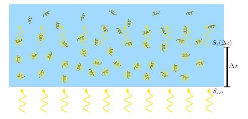
**Figure 5.7:** Sketch of the proposed angular independent polarization filter. The filter consists of a slab with randomly oriented and randomly placed optimally designed helices. Because the averaged absorption cross section of the helices is different for illumination fields of different helicities, the decay of the field along the slab will be more pronounced for one of the illumination fields.
