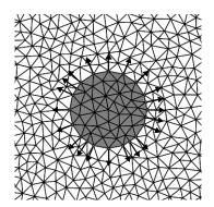
**Figure 2.5:** Calculation of the shape derivative of the finite element discretization with respect to the radius of the circle, *R*. The change in the radius imply a change of the position of the vertices that compose the boundary of the circle. The calculation of the shape derivatives of the mesh discretization is one of the main steps necessary to compute the shape derivatives of the electromagnetic field with the finite element method.
