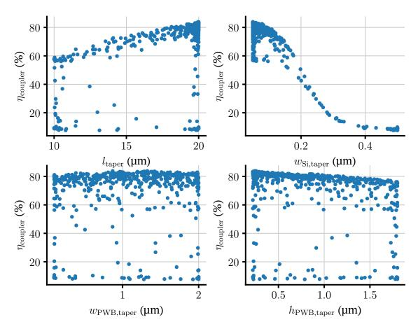
**Figure 5.17:** Optimization results for the waveguide coupler. Projections of the coupling efficiency over the different parameters of the design space. The parameters are defined in the schematic of Fig. 5.11. Note that the difference with the reuslts shown in Fig. 5.13 is the different search range for the parameter  $l_{taper}$ .
