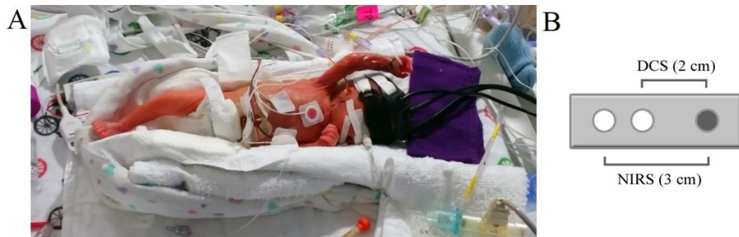
Figure 4.1: A) Premature infant with optical probes secured to the forehead and phototherapy eye shield, B) schematic of probe holder with NIRS (3-cm SDD) and DCS (2-cm SDD) optical fibers with the common detection fiber shaded; probe holder dimensions: 5×2×1 cm.
