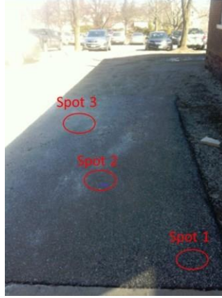
Fig. 20 Asphalt Pavement Dielectric Constant Monitoring Test Spots
