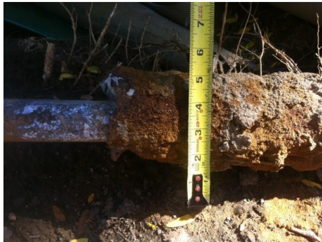
Figure 43 An excavated pipe which was consistent with the GPR result in Figure 34
