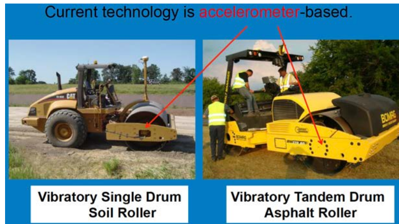
Figure 3. Accelerometers mounted on the rollers (Source: Naras et al., 2015)
