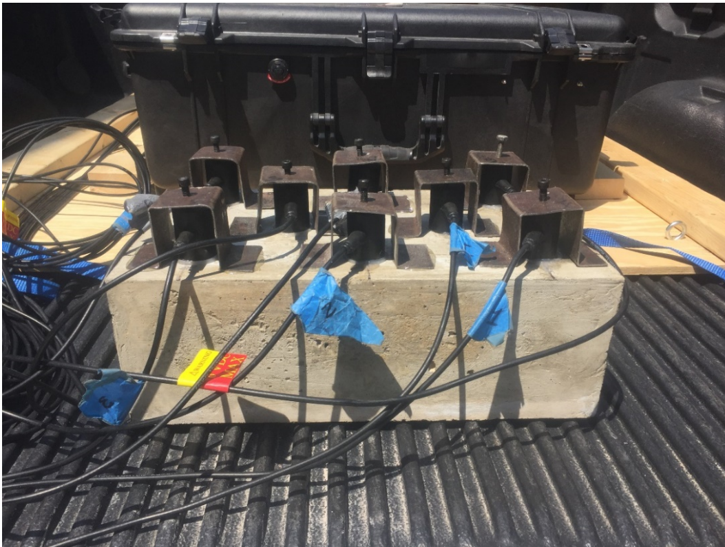
Figure 7.2 AE sensor connection to concrete block with U-shape brackets
