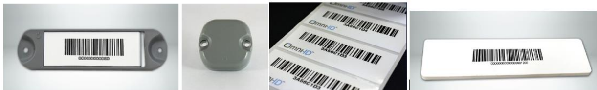
Fig. 16. RFID tags used in the experiment. (From left to right are tag 6 (Omni-ID Flex 800), tag 14 (Omni-ID Exo 750), tag 12 (Omni-ID IQ 800), and tag 7 (Omni-ID Flex 1200).)
