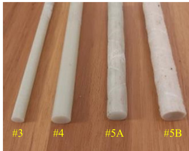
Fig. 3-1. GFRP bars used for creep rupture tests.
