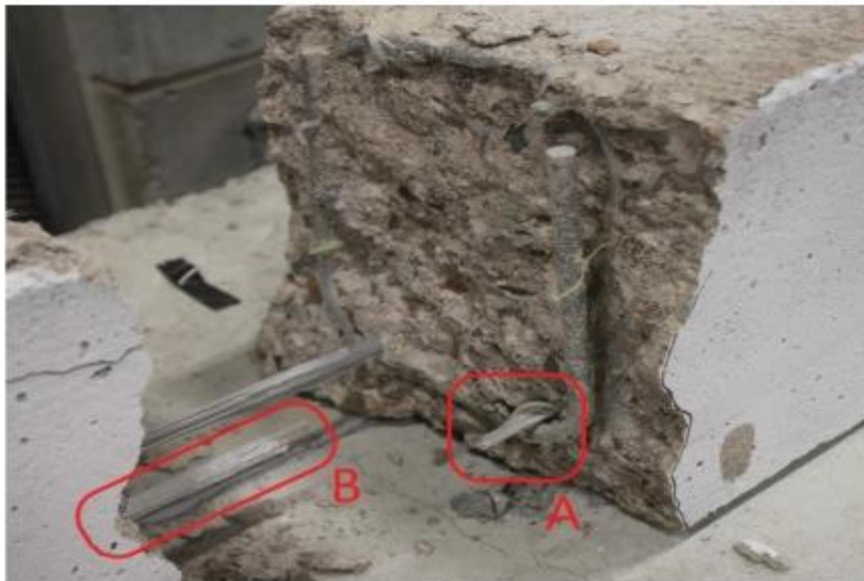
Fig. 4-9. Failure mode of GFRP bars in an aged beam
