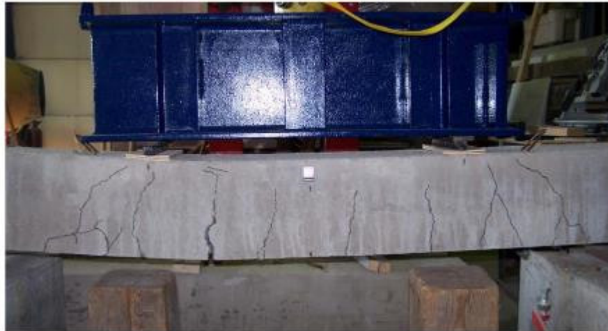
Fig. 4-7. Typical failure of the unconditioned beams
