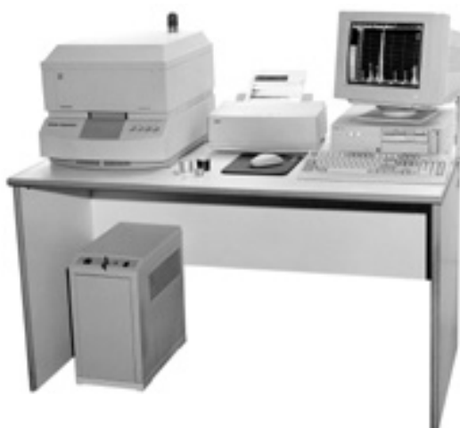
Figure 6. Spectron-Optel RMA WD-XRF spectrometer (photo: B. Igliński)
