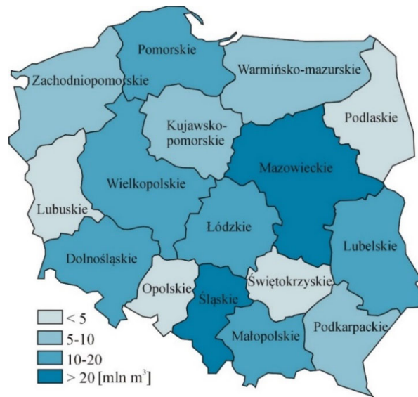
Figure 11. Volume of BM that can be obtained for municipal waste in Poland (mln m 3 /year).
