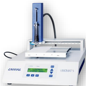
Figure 1.4 Scheme of the instrument Linomat 5 (adapted from CAMAG 93 ).
