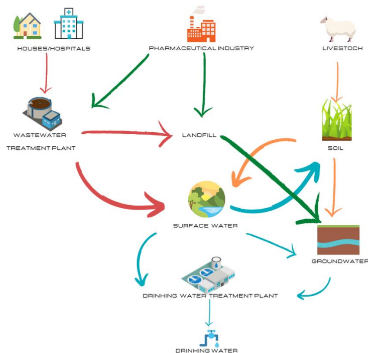
Figure 3.1 – Representative sources and routes of estrogens in the environment (adapted from Adeel et al., 2017; Barbosa et al., 2016)
