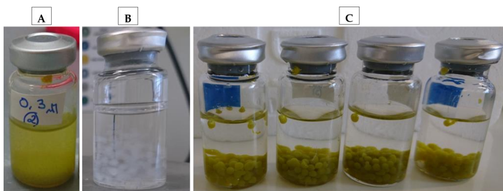
Figure 3.29.- Desulfovibrio desulfuricans -CdS-MoS 2 system in suspension (A) vs. immobilized (C) in calcium alginate beads (B).
