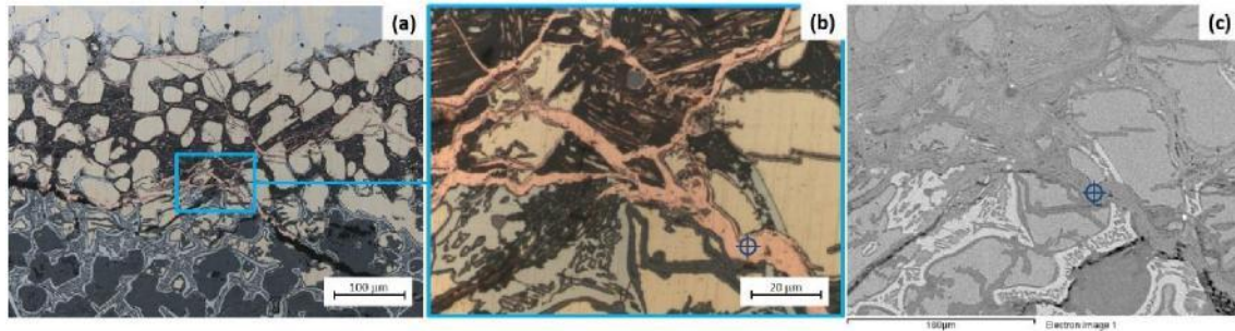
Fig. 11. (a) Detailed OM bright field image of sublayer 2b of Famalicão cross-section, showing corroded \delta -phase (black coloured) and redeposited metallic copper (pink) in the available spaces (200 \times ). (b) Higher magnification OM bright field image of the area marked in the previous image (1000 \times ) and (c) BSE-SEM image obtained in the same area showing redeposited copper in the interface between sublayers 2a and 2b. An analyzed spot (99.1 at.% Cu) is depicted with a target in (b) and (c).
